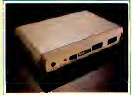
Interface devices are necessary in order to use a printer or modem.
